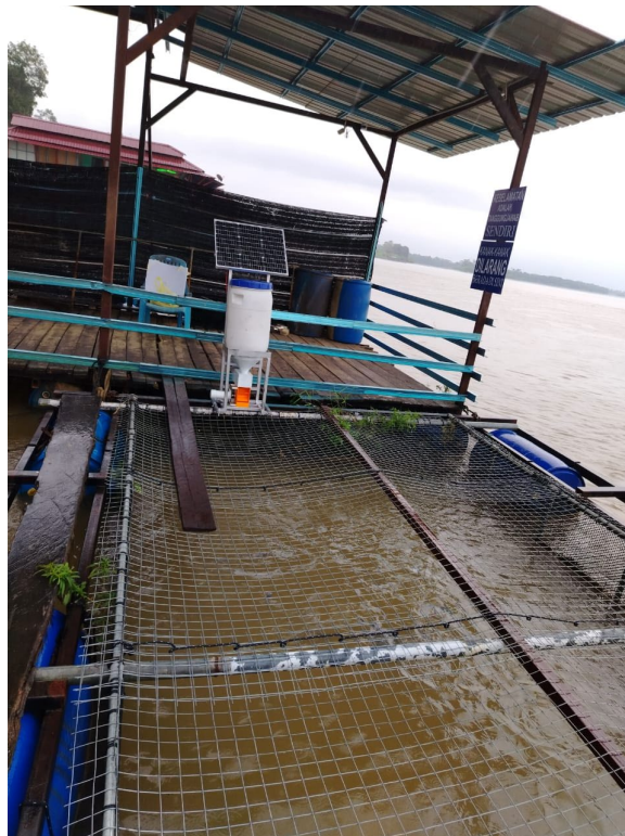
Figure 1. Automatic feeding system, integrated as a core component of the iSENSfishery smart aquaculture platform.
