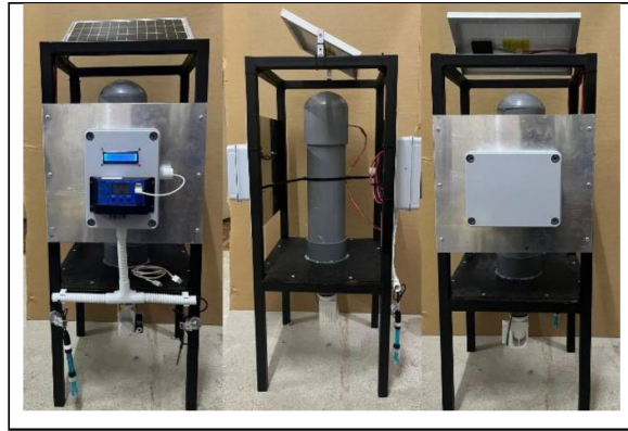
Figure 4. Complete hardware setup of the intelligent aquaculture monitoring system, integrating IoT sensors, ESP32 microcontroller, LCD display, and automated control components for real-time water quality management.
