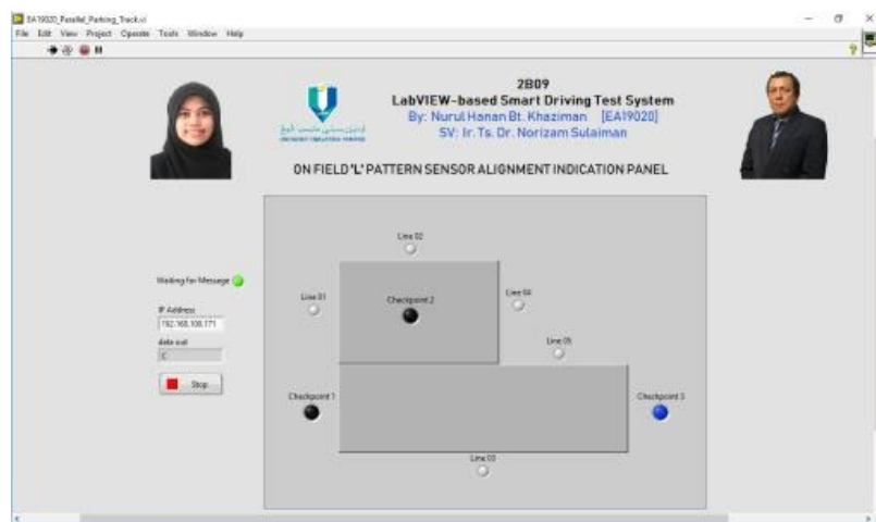
Figure 20. LabVIEW GUI for the L-shaped parking test at checkpoint 3
